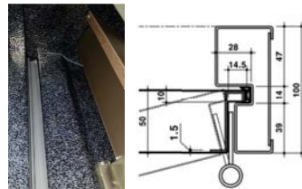
Door is combined to the hole of hinge bar , which strengthen the fire rating function.
